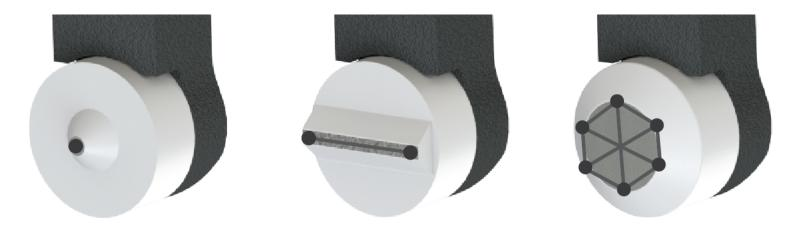
✓ Kinematic constraints from different contact geometries.
