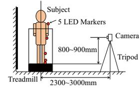
Fig. 1. Walking measurement system
