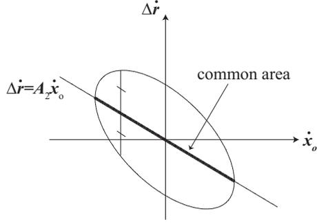
Fig. 2. Mapping of the ellipsoid onto  $\dot{x}_o$  space
