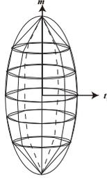
Fig. 4. Linearized frictional tangential forces and moment around the contact normal direction
