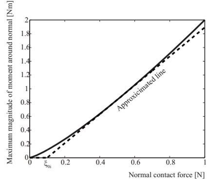
Fig. 3. Relation between maximum moment around contact normal and normal force (tangential force is zero and  $\mu_{mi} = 2$ ,  $\gamma = 0.25$ )
