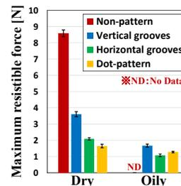
Fig. 8. Maximum resistible force when grasping a silicone cube by the fluid fingertips under dry and oily conditions
