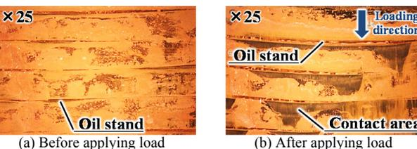
Fig. 17. Contact area of the horizontal slits before and after applying a load under the oily condition; the oil is colored in red.
