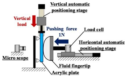
Fig. 13. Schematic view of the experimental setup for observing the contact area
