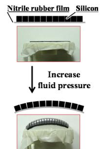
Fig. 9. Arrangement change by increasing fluid pressure
