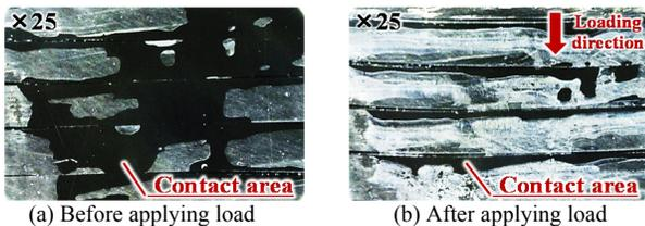
Fig. 15. Contact area of the horizontal slits before and after applying a load under the dry condition
