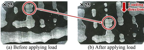
Fig. 14. Contact area of the non-pattern before and after applying a load under the dry condition
