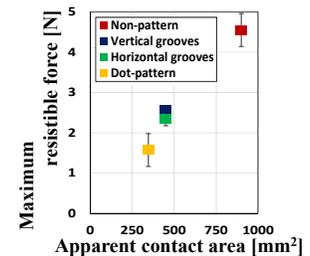
Fig. 6. Relationship between the apparent contact area and maximum resistible force when grasping a silicone cube by the rigid and flat plates under dry conditions
