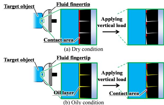
Fig. 12. Hypothesis of local surface deformation for the horizontal and grid slit texture patterns
