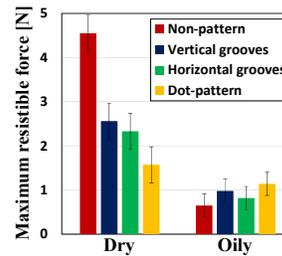
Fig. 5. Maximum resistible force when grasping a silicone cube by the rigid and flat plates under dry and oily conditions
