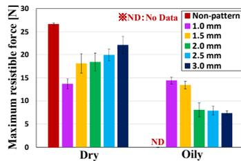
Fig. 23. Maximum resistible force for the concentric hybrid texture pattern
