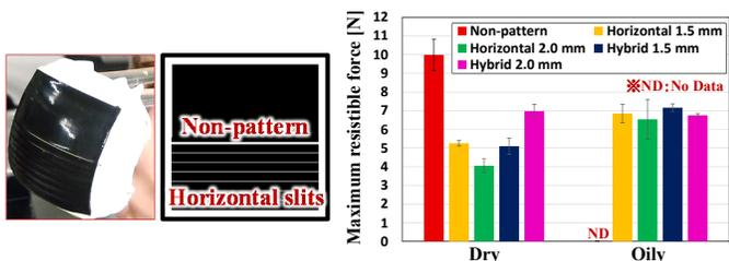
Fig. 20. Fluid fingertip with a hybrid texture pattern of non-pattern and horizontal slits
