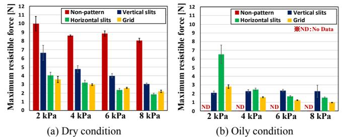
Fig. 11. Maximum resistible force for various fluid pressures and various slit texture patterns
