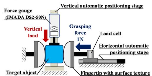
Fig. 4. Schematic view of experimental setup for resistible force test
