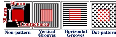
Fig. 7. Schematic view of the apparent contact area for each texture pattern
