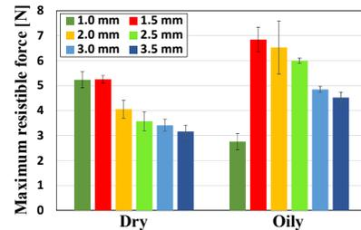
Fig. 18. Maximum resistible force for various slit intervals; the horizontal slit texture pattern with a fluid pressure of 2 kPa was evaluated under dry and oily conditions
