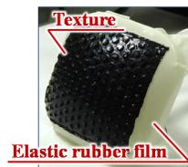
Fig. 1. Fluid fingertip with surface texture
