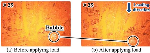
Fig. 16. Contact area of the non-pattern before and after applying a load under the oily condition; the oil is colored in red
