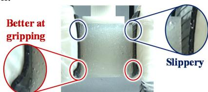
Fig. 19. Side view of the object grasped by the fingertip with the horizontal slit texture patterns after applying a load under the oily condition; investigation of how the slit interval changed with loading
