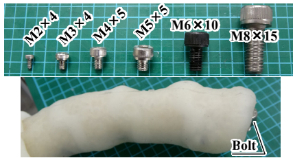
Figure 18. Target objects and overview of the grasping test utilizing the fingertip as a jamming gripper.
