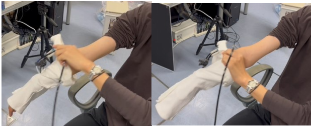
Figure 5. Shape of the developed sleeve during undressing (Left :without air pressurization, Right: with air pressurization)
