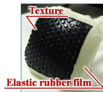
Fig. 1. Fluid fingertip with surface texture
