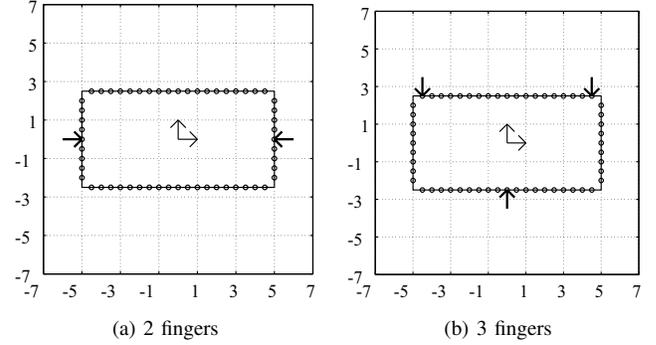
Fig. 7. Optimal grasp points in Case I
