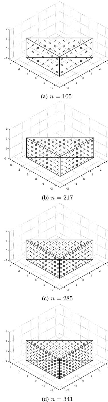
Fig. 11. Target object and candidate contact points for various  $n$ 's
