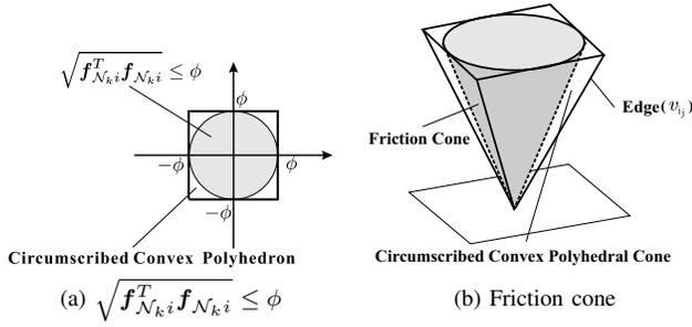
Fig. 2. Convex polyhedron and convex polyhedral cone circumscribed in the constraints of Subproblem2
